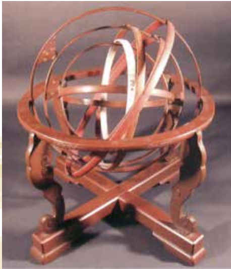
Armillary sphere model used at Shiko (an armillary sphere is used to measure and determine positions of heavenly bodies)
